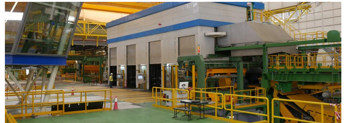
Four-stand Tandem hot finishing mill - Aluminium segment
